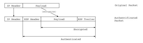
IPsec: The transformation of an packet to an encrypted one.
