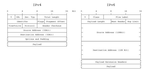
The header structure of IPv4 faced against IPv6's ones.
