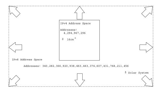
Analogy IPv4 to IPv6 Address Space compared with  $16cm^2$  to area of solar system
